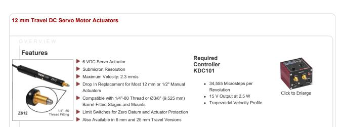
These Motorized Actuators are engineered for use with optical positioning devices. They offer high resolution in a lightweight package, which makes them ideally suited for demanding optical laboratory automation applications. The Z812 delivers 12 mm of travel and has been designed as a replacement for the former-generation Z712 motor.
